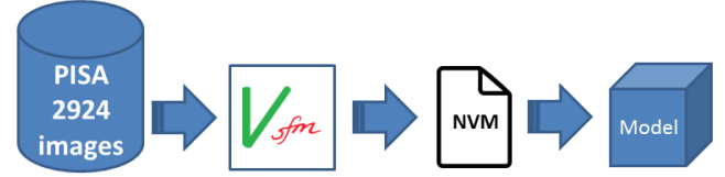
Figure 1: Initial workflow: images of a collection are processed with VSfM and a Model is obtained through parsing of the NVM file (3D reconstruction) and meta-data aggregation from our framework.
