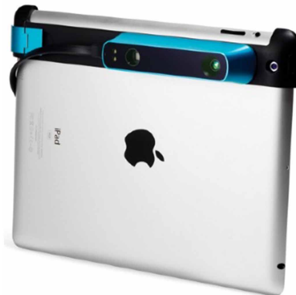
Figure 7. Structure Sensor clipped on the iPad
