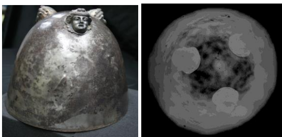
Fig. 5. X-Ray acquisition on Mastòs (NI 9): upper-lower projection
